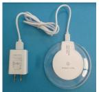
Connect the power adapter to an AC outlet and the diode on the charger station illuminates red.
